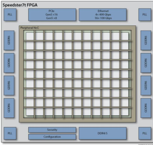
Fig. 3. External interfaces of Achronix Speedster7t FPGA
