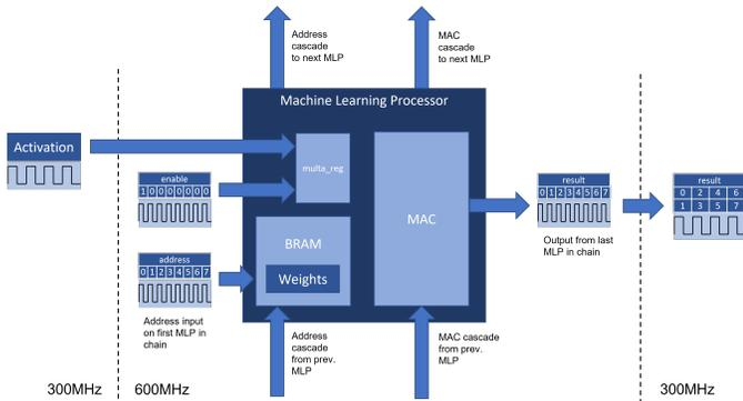
Fig. 6. Double Clocking Scheme for MAU Core Architecture on Achronix Speedster7t FPGA
