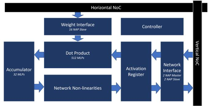
Fig. 5. The MAU Core Architecture on Achronix Speedster7t FPGA
