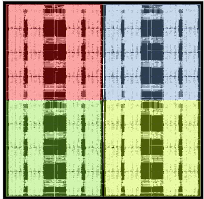
Fig. 7. Floorplan of dot product circuit on Achronix Speedster7t FPGA
