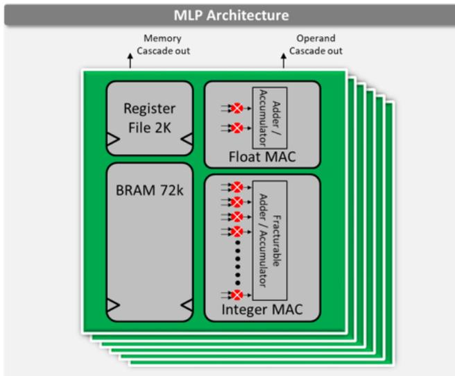
Fig. 1. MLP Architecture on Achronix Speedster7t FPGA
