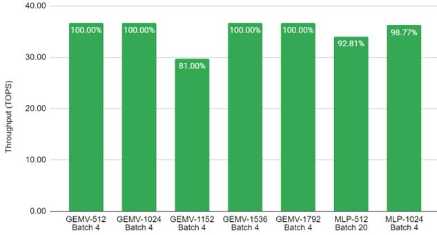
Fig. 8. Throughput of key AI Benchmarks on Achronix S7t-VG6 VectorPath Accelerator Card. Results were measured on a C2 speed-grade device at 560 MHz. Labels show utilization as a percentage of the headline performance of the MAU Accelerator®.
