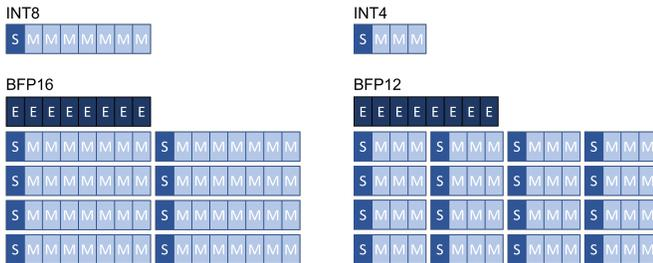
Fig. 2. Block Floating Point Quantization Format
