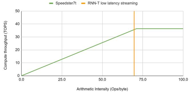
Fig. 9. Achronix Roofline Performance and RNN-T operating point, using headline memory bandwidth
